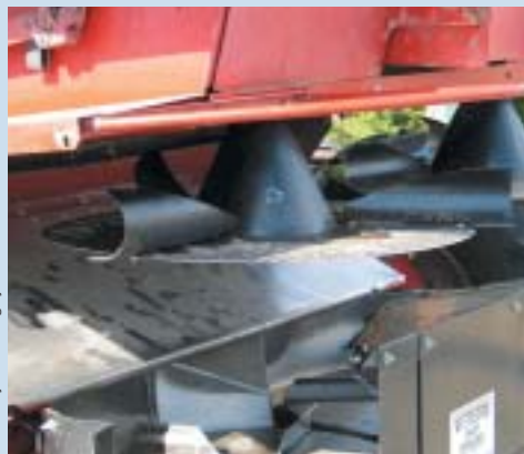
CIH with more aggressive bats installed.
