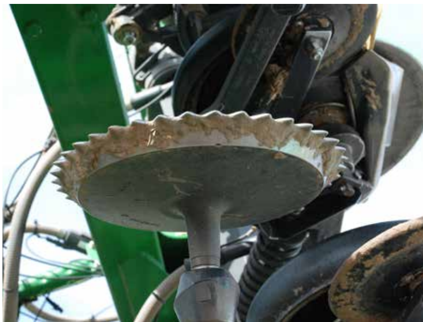
Joe Swanson is testing a 38-tooth add-on closing wheel made by Mark Vogts of Hillsboro, Kan. Made from quarter-inch plate, the wheels bolt onto the factory cast iron wheels, letting growers use original equipment. They cost $50 each, including replacement bolts and nuts.
