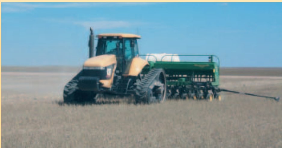
Maskus seeding wheat Sept. '05 using a neighbor's 20-ft. 750 on 7.5-inch spacing.
