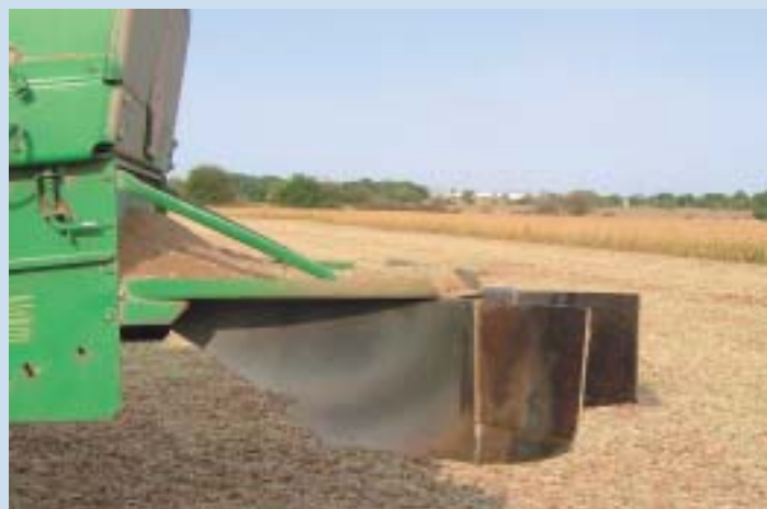
Farmer-built extensions for the chopper vanes.
