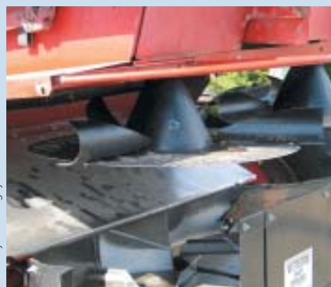
CIH with more aggressive bats installed.
